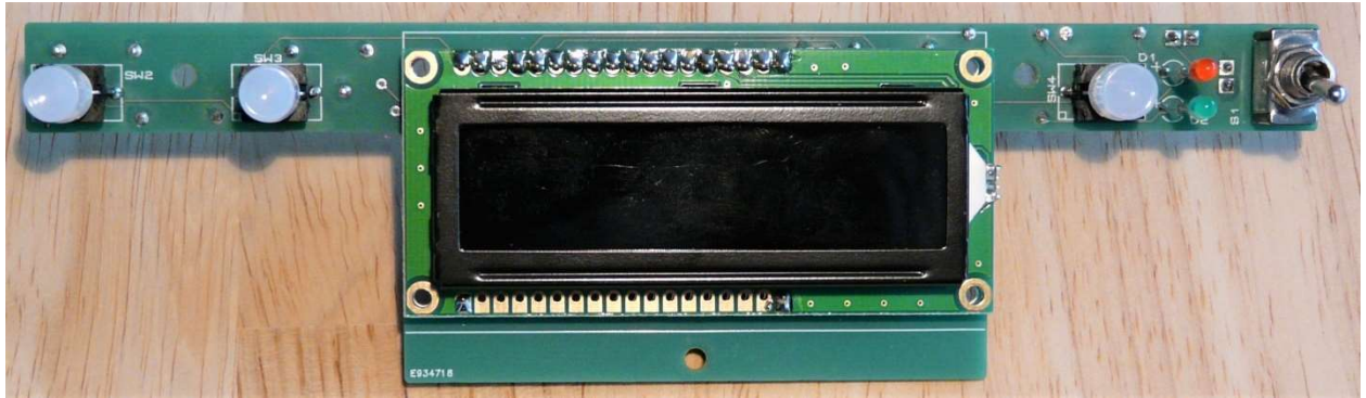
Figure 5 – completed front side display & control board
