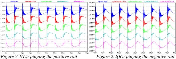
Figure 2.1(L): pinging the positive rail with 100kHz 0 to +10mA square wave, 5mV/div, traces spread by 10mV
