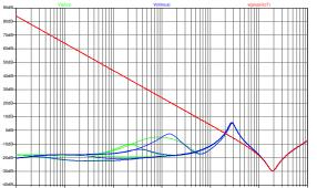
Figure 2.5(L): rail impedance as we increase the regulator output cap from 2.2uF up to 2200uF, decade steps. This is with the noise bypass caps.
