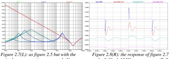
Figure 2.7(L): as figure 2.5 but with the noise bypass capacitors removed. Note the resonant peak in the audio band
