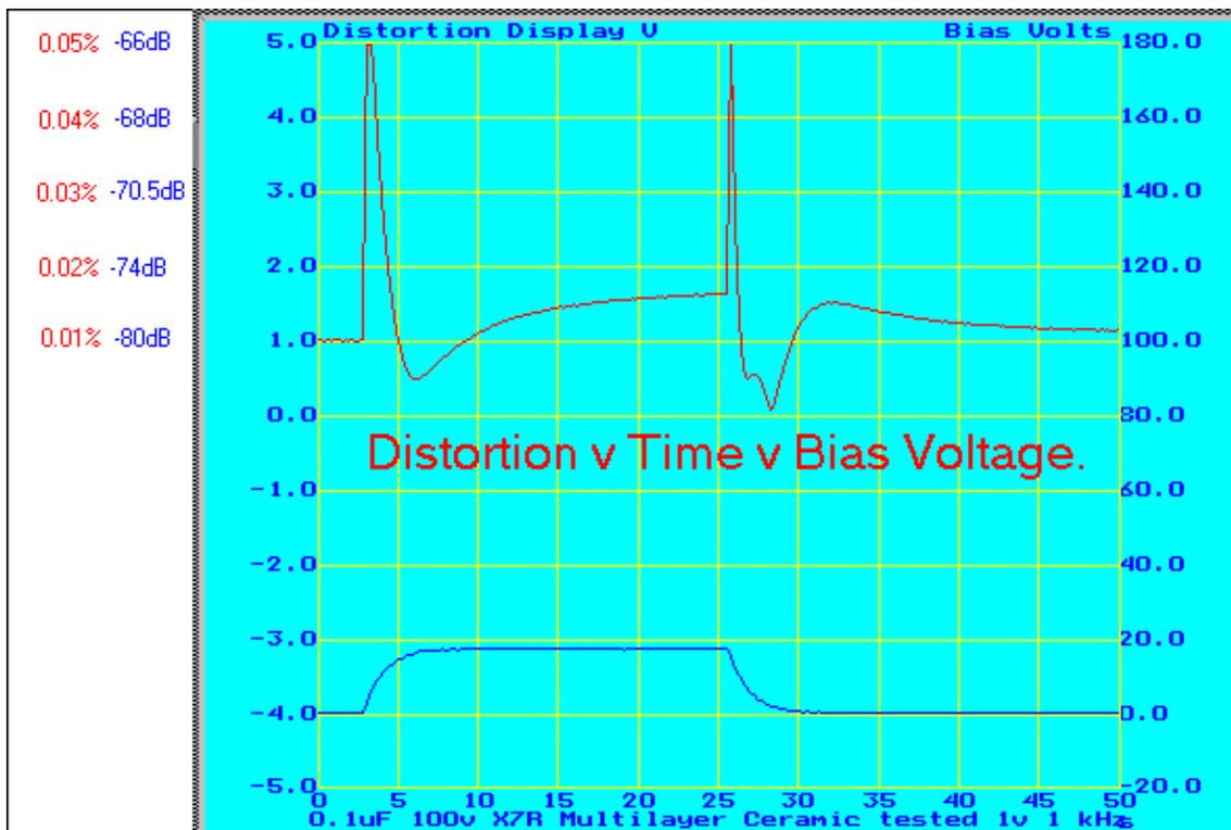
**Figure 1)** The top plot, left scale, of a 0.1µF X7R multilayer ceramic, shows second harmonic distortion both increasing and reducing prior to a prolonged settling period, in a capacitor having 1.76% dielectric absorption. This anomalous behaviour was hidden using the soundcard / software method. Bottom trace, right scale, shows DC bias voltage as measured across the capacitor.
