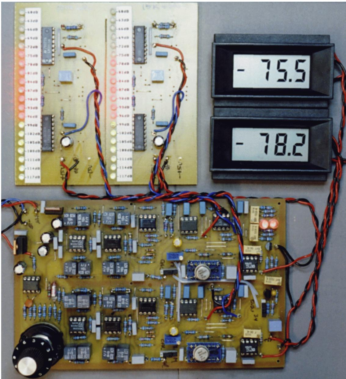
**Figure 4)** The real time hardware on initial tests, shows good agreement between the two LED tree displays and the two DMM displays.
