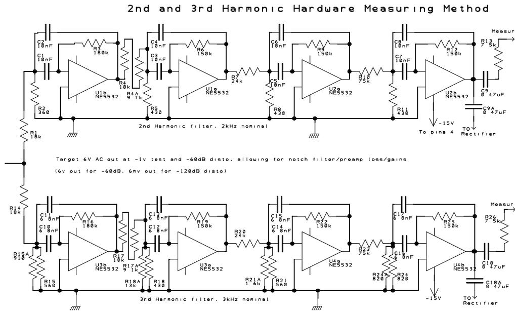
**Figure 5)** MFB second and third harmonic filters have low noise, low distortion and high rejection of unwanted signals, responding accurately to distortions down to -120dB, in the presence of the much larger fundamental test frequency.
