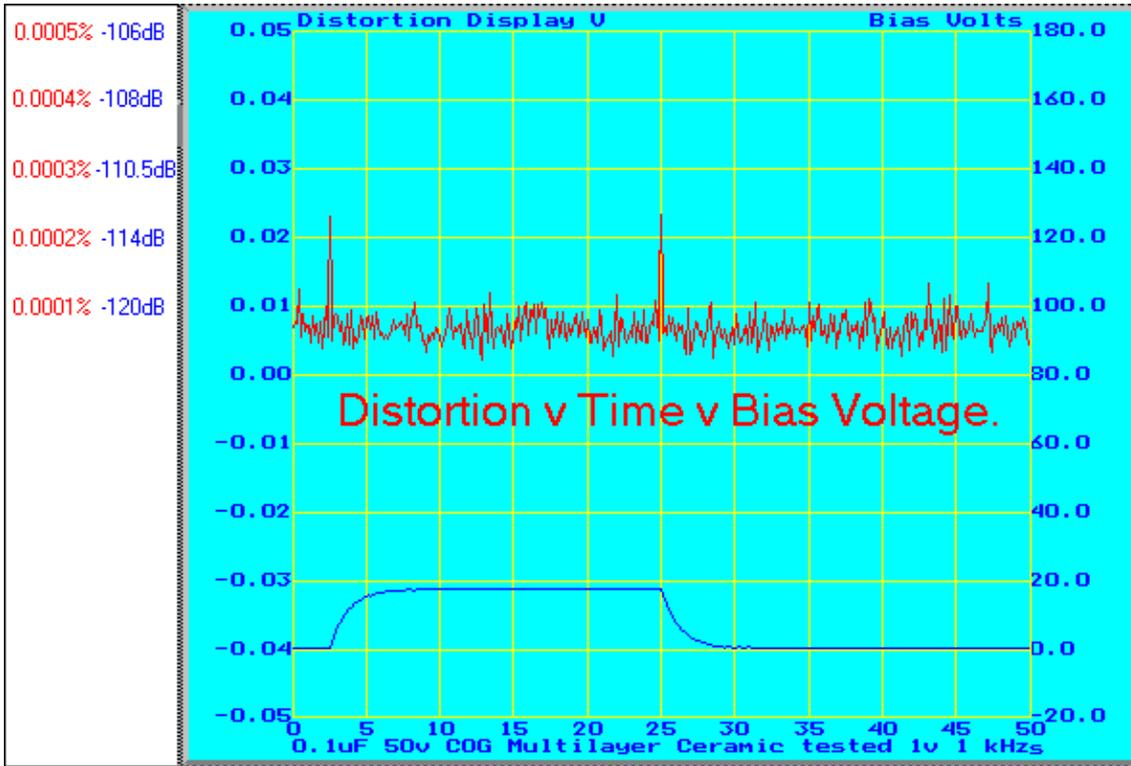
**Figure 2)** This distortion plot of a 0.1µF COG multilayer ceramic, scaled 100 times more sensitive than Figure 1, was made a few seconds later.
