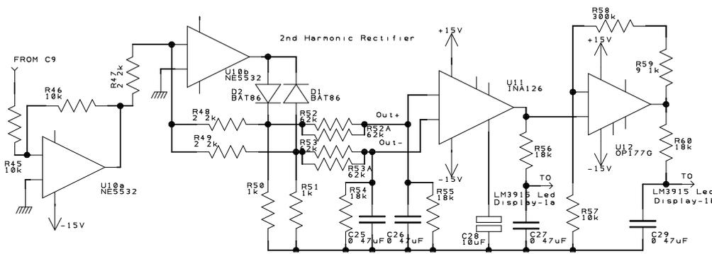
**Figure 6)** The full wave rectifier used to drive 10 volts DC to an LM3915 for -60dB full scale distortion, is driven from a low source impedance, unity gain inverting buffer.
