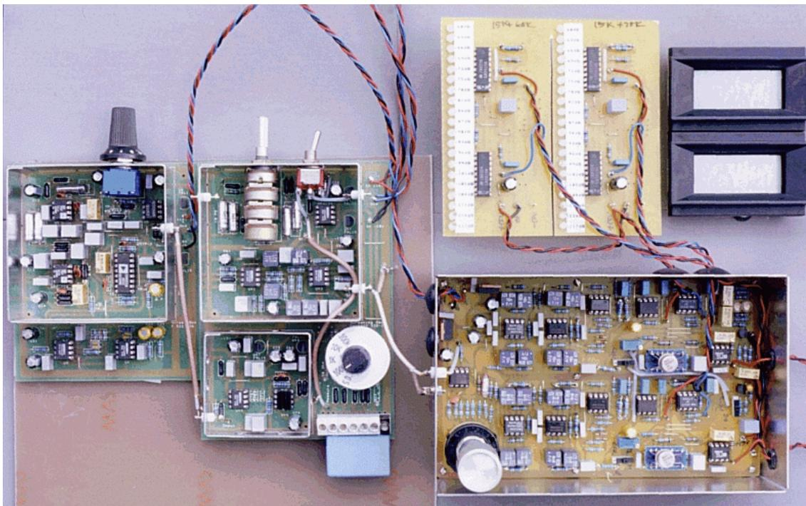
**Figure 3)** The full measurement set-up less screening lids, as used for Figures 1 & 2, shows this new real time hardware connected to my notch filter / preamp described in the capacitor sounds series.
