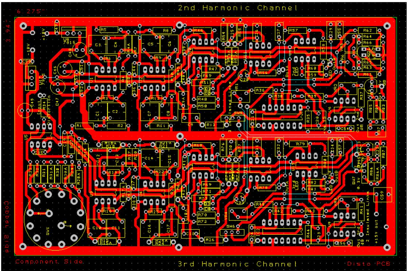
**Figure 9)** The main PCB used for the prototype assembly shown. This board houses the complete real time distortion measurement system but the forty display LED's and their LM3915 logarithmic display drivers were located on two small, low density, panel mounting PCB's.
