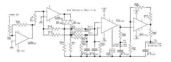
Figure 6) The full wave rectifier used to drive 10 volts DC to an LM3915 for -60dB full scale distortion, is driven from a low source impedance, unity gain inverting buffer.
