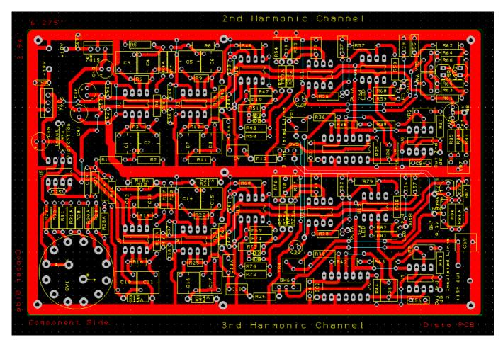
**Figure 9**) The main PCB used for the prototype assembly shown. This board houses the complete real time distortion measurement system but the forty display LED's and their LM3915 logarithmic display drivers were located on two small, low density, panel mounting PCB's.
