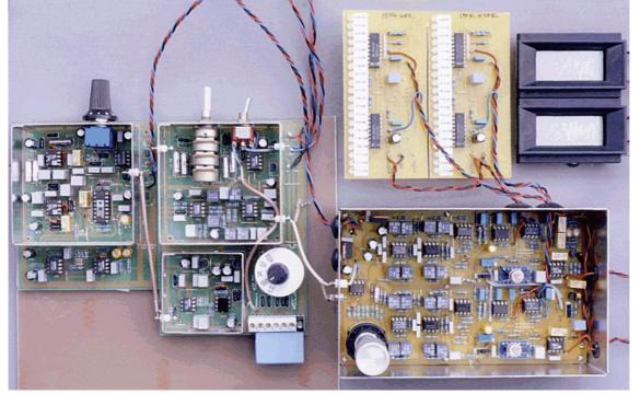
Figure 3) The full measurement setup less screening lids, as used for Figures 1 & 2, shows this new real time hardware connected to my notch filter / preamp described in the capacitor sounds series.
