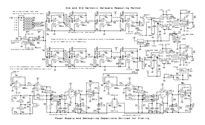
**Figure 8)** The schematic of the prototype assembly, less supply and decoupling capacitors omitted for clarity. Six Rubycon 100  $\mu$ F 25 volt YXF electrolytics with twenty three BC Components 0.1 $\mu$ F 63 volt type 470 metallised PET, decoupling capacitors and two 15v stabilisers were used.
