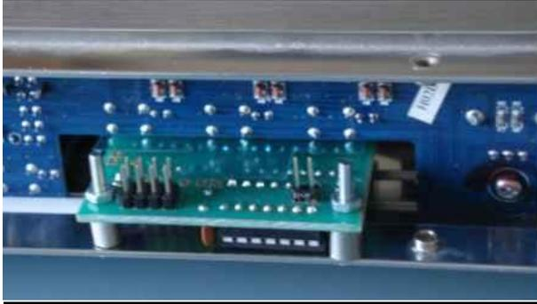
Next, carefully mount the display/control board with the included 2.5mm hardware and the 8mm stand-offs. It should look like the pic to the left. The display should just touch the Plexiglass window at the front. Double-check that the board is not bent or anything and that there are no obvious shorts or mechanical problems. Note the plastic sheets and the reverse-mounted J1, J7.
