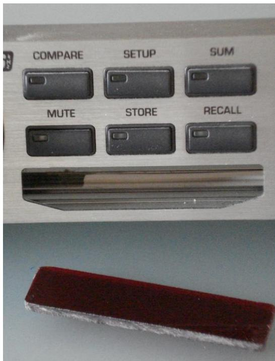
Now check the front panel from the inside to where the bezel has been and where the red Plexiglass window needs to go. If there is still some remaining glue around the edges, use a pair of tweezers and/or a small knife to clean that up. The pic on the left shows the DCX front panel assembly with the card slot bezel removed and the small red Plexiglass window to be mounted on the inside, which is included in the kit.
