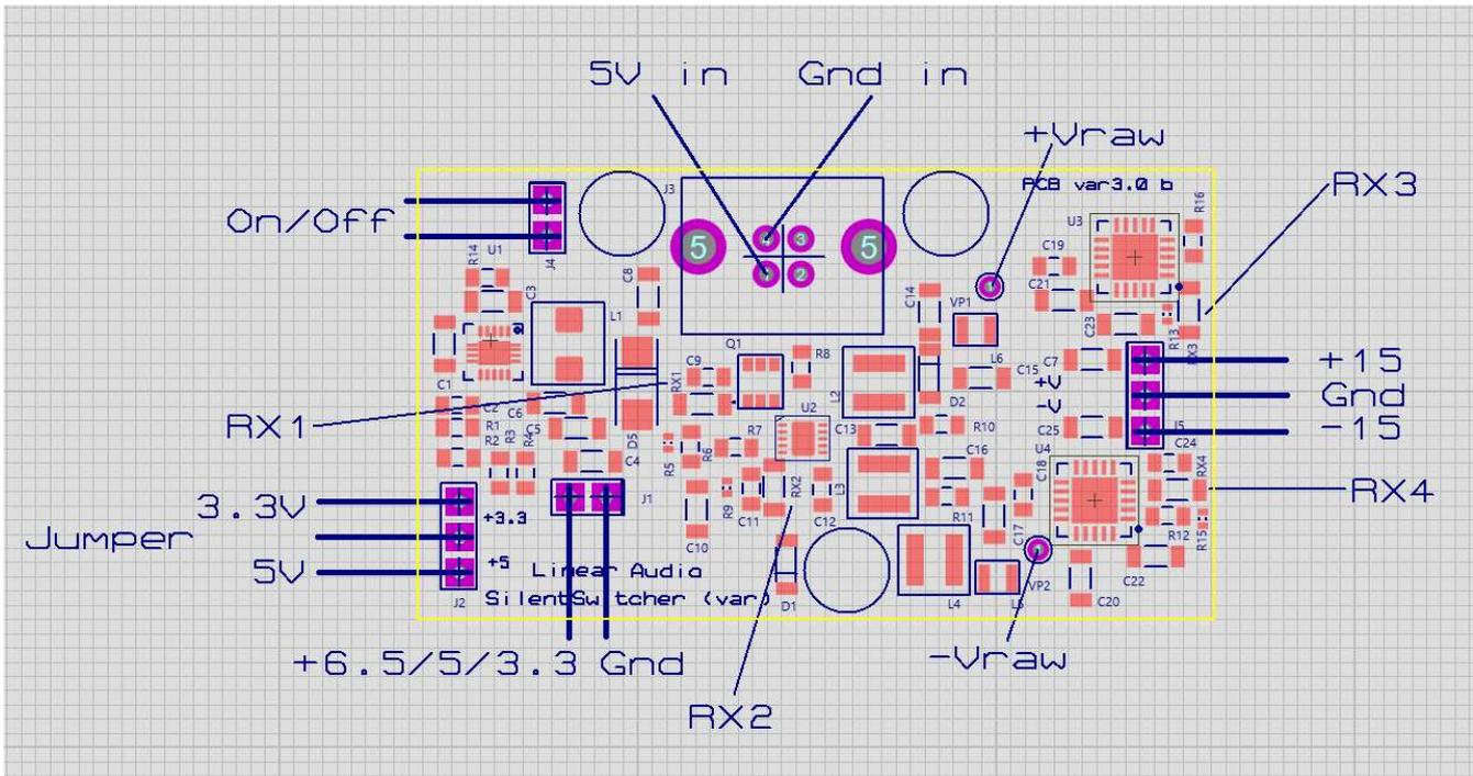
Figure 1 – resistor locations and test points
