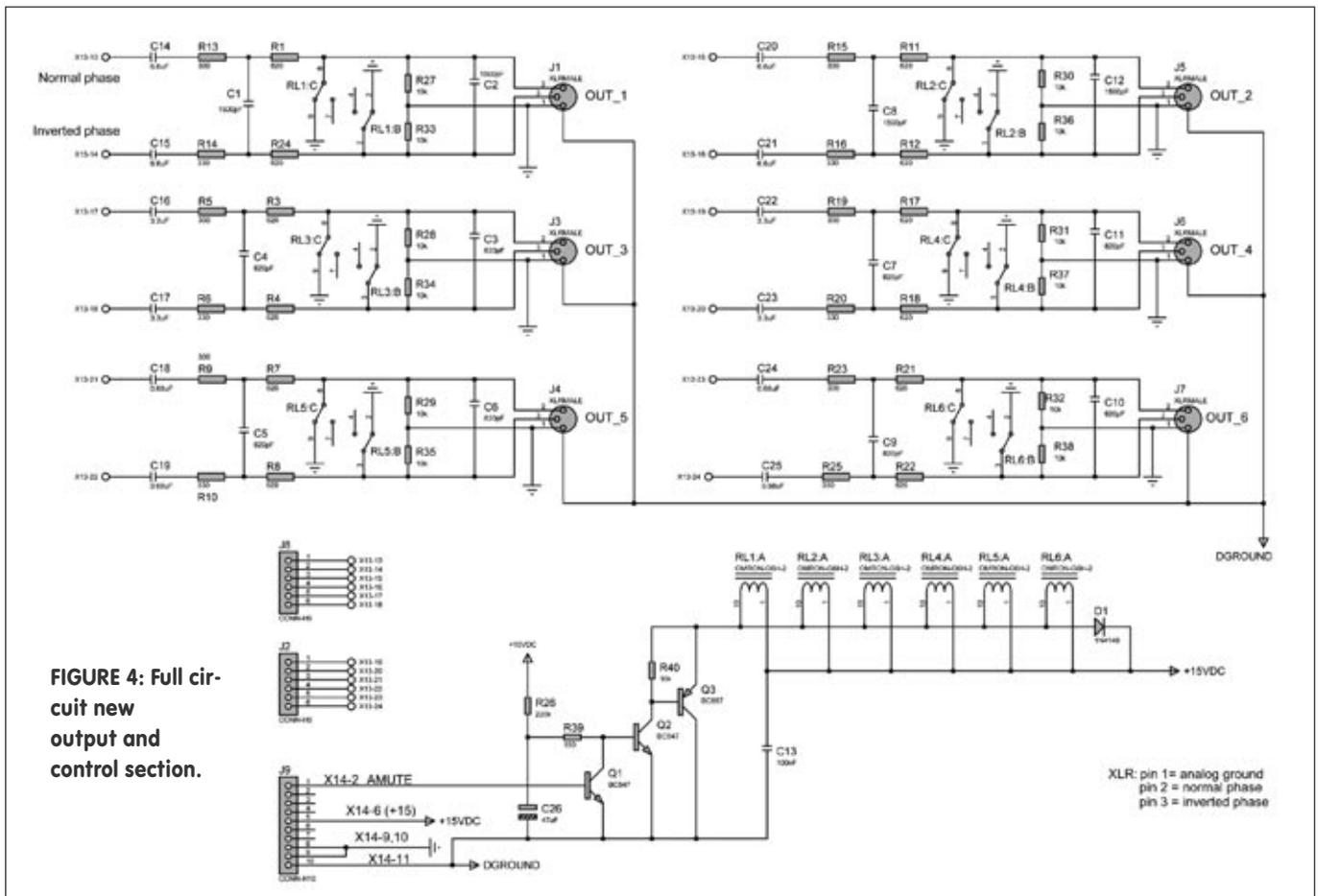
**FIGURE 4: Full circuit new output and control section.**
