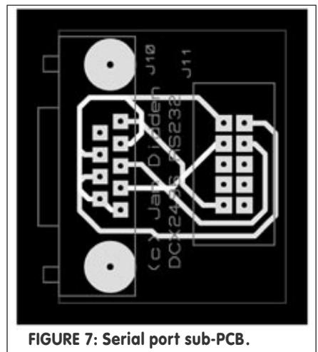
FIGURE 7: Serial port sub-PCB.
