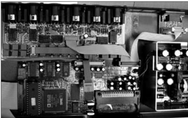
PHOTO 1: Cable layout with new board installed.
